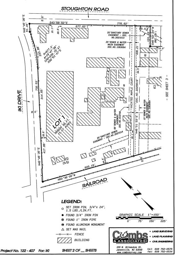
PART OF OUTLOT 9, ASSESSOR'S PLAT OF THE CITY OF EDGERTON AND PART OF VACATED MAPLE CT.& ST. (DOC.NO.1856610 & 2225619) AND VACATED W. ROLLIN STREET (DOC.NO.1856610), ALL BEING LOCATED IN THE SW 1/4 OF THE NE 1/4, NW 1/4 OF THE SE 1/4, NE 1/4 OF THE SW 1/4 AND SE 1/4 OF THE NW 1/4 OF SECTION 4, T.4N., R.12E. OF THE 4TH P.M., CITY OF EDGERTON, ROCK COUNTY, WISCONSIN.
